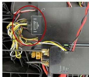
20、 One end of the wiring harness from the FC interface of RTK is connected to the main control, and one end is connected to the 12V interface of the radar module.
