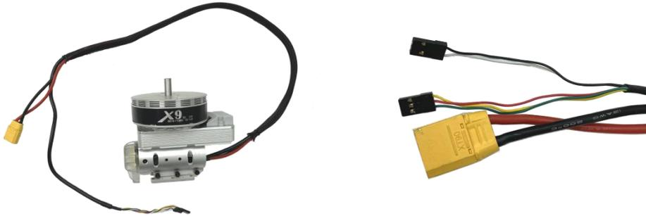
5. Put the motor harness into the snakeskin net tube and weld the XT90 male connector, paying attention to distinguish the positive and negative poles. (It is recommended to use small cable ties to tighten the ends of the snakeskin net tube to avoid the snakeskin net tube from branching.)
