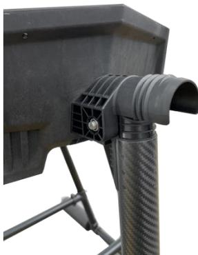
9、 Install the front and rear arm components: use M8\*65 round head screws to fix the front and rear carbon tube arm components ( $\phi 40 \times 520$ ) in the front and rear threaded parts.
