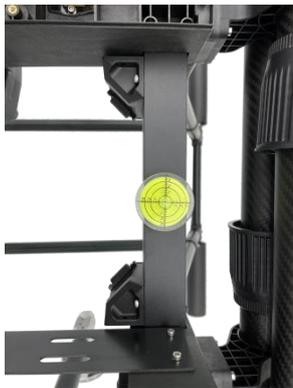
10 、 Calibrate the body horizontally. Adjust the body level until the display is centered. If it is not level.
