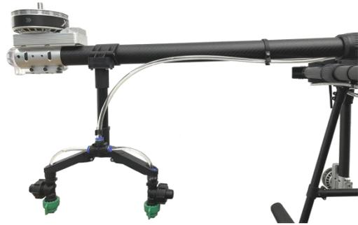
13、 Water pipe installation: connect the water pipe to the extension rod Y-type double nozzle T-type tee.
