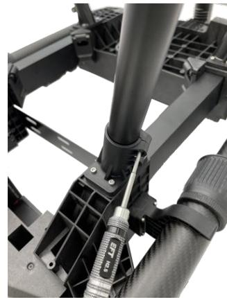
6. After the diagonal brace installed, tighten the M3\*12 screws of the tripod fixing seat.
