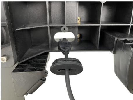
11、Pass the radar harness through the seal of the front fuselage to the inside of the fuselage.
