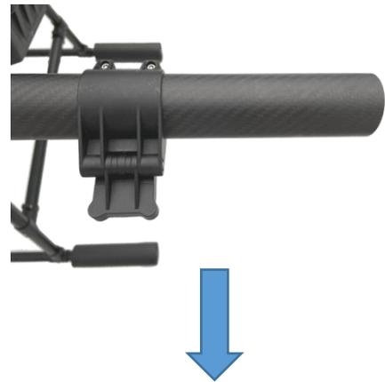
4. Set the spray rod fixing components into the left and right arms (note that the installation direction requirements: buckle the left and right 4 arms in the arm pipe clamps, rotate the spray rod rotating parts in place, and require the end of the spray rod rotating parts to point to the fuselage. On the outside, the flat side of the spray rod rotating part is parallel to the ground, and the spray rod fixing part assembly should be as close as possible to the end of the machine arm).
