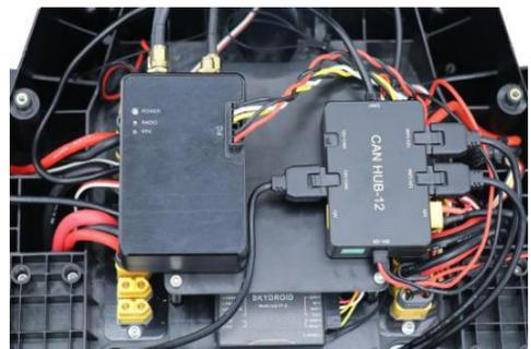
18、 Use 3M glue to fix the RTK and radar module on the flight control mounting board.
