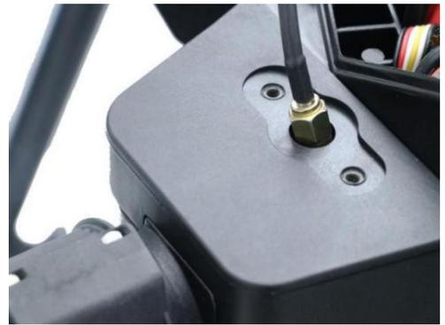
16、 The RTK antenna needs to pass through the reserved hole to reach the flight control compartment.
