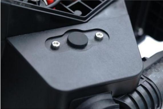
15、 There are reserved holes for the RTK antennas at both ends of the front fuselage.
