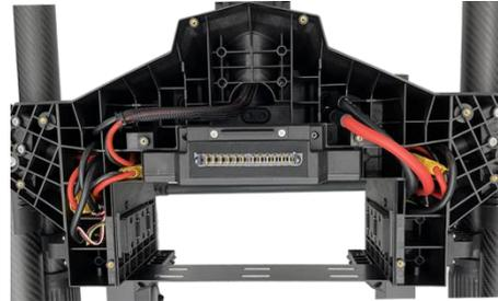
9、 Installation drawing of the power harness of the rear fuselage.
