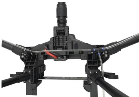
10、 Water pipe installation: As shown in the figure, the water pipe leading from the cross beam to the rear fuselage leads to two water pipes through the pneumatic tee to reach the arm where the No. 3 and No. 5 motors are located.
