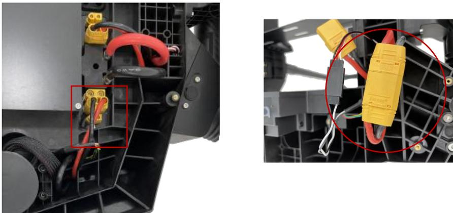
7. The XT90 plugs of the wiring harness (No. 1, No. 2, and No. 6 motors) are directly inserted into the plug of the distribution board, and the XT90 plugs and ESC signal wires of the wiring harnesses of the No. 3, 4, and 5 motors are respectively inserted into the reserved wiring harness. Pay attention to distinguish the CW /CCW motor. (The flight control cabin is the direction of the nose).
