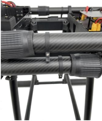
1. Put the water pipes into the left and right arms.
