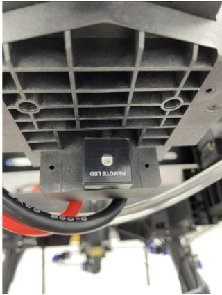
9、 The LED light installation: Use 3M glue to fix the LED light on the patch position at the bottom of the tail.
