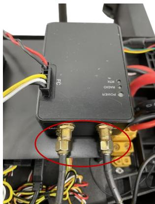
19、 The antenna harness is connected to the RTK.
