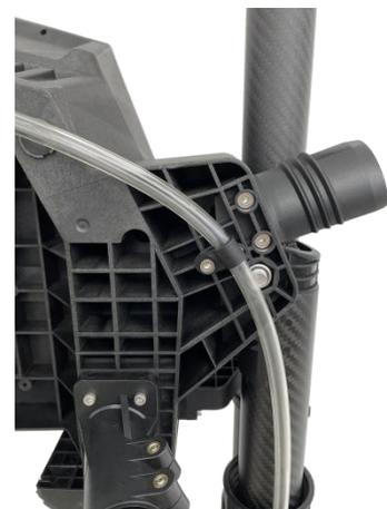
11、 Water pipe installation: the water pipe from the water outlet of the water pump needs to pass through the R-type water pipe clamp.
