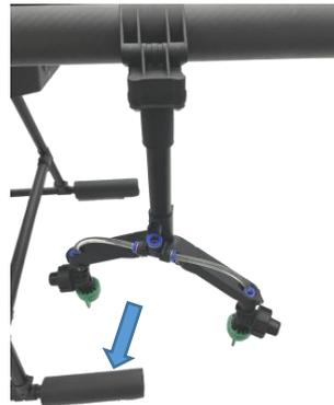
3、 Use M3\*16 cup-head self-tapping screws to fix the Y-type double nozzle on the rotating part of the spray rod. (Note that the Y-type double nozzle has a direction requirement: buckle the 4 left and right arms in the arm pipe clamps, there are 6- 8-6 pneumatic tee should point to the outside of the aircraft).
