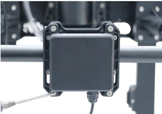
9、 The radar fixing plate installation : This is the installation method of ground defense radar, which can be directly fixed with M4\*10 self-tapping screws.
