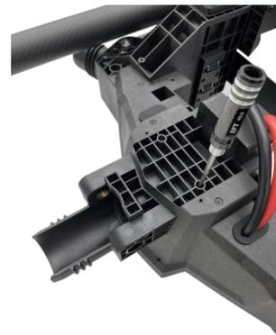
8、 Install the front and rear threaded disassemble components: Align the screw holes and use 2 M3x10 screws to fix the lower part.
