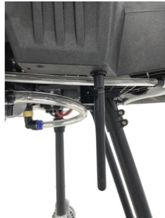
5、 The H12 receiver antenna installation: remove the waterproof ring of the fuselage, and the antenna can be fixed in the reserved hole of the fuselage.
