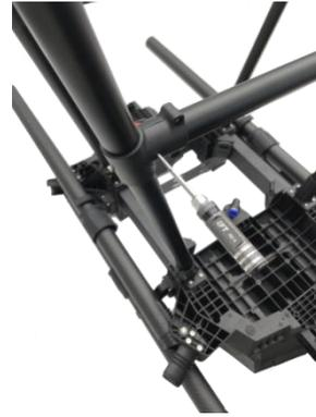
4. Install the radar pole: insert the radar crossbar into the diagonal tee, fix the back limit screw, and then fix all the screws of the oblique tee.
