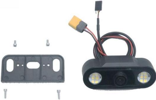
1、 Camera adapter: Use M3\*6 screws to fix the camera in the adapter plate, and then use M3\*10 self-tapping screws to fix the camera adapter on the body.
