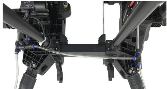
9、 Water pipe installation: Insert an 8MM water pipe into the 8MM interface of the 8-10-8 pneumatic tee, as shown in the figure, and lead the water pipe from the front fuselage to the rear fuselage.
