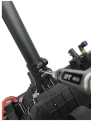
3. Install diagonal brace: Put the aluminum tube with limited hole end into the tripod fixing seat and reach the deepest part of the fixing seat. Use M3x10 cup head limit screws to fix the diagonal brace.
