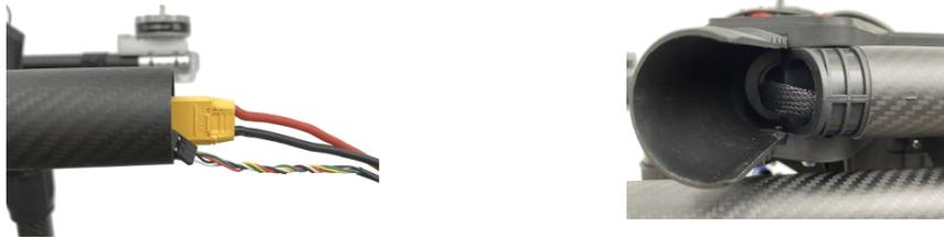
6. Install the power in sequence according to the direction of the machine head, and pass the motor harness through the machine arm to the inside of the machine body. Pay attention to distinguish the CW/CCW motor.
