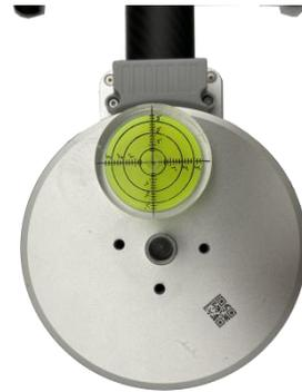
11、 Fully unfold the arms after adjusting the fuselage, tighten the nuts, and perform horizontal motor calibration. The calibration method is the same as that of the fuselage, and fix the motor screws.
