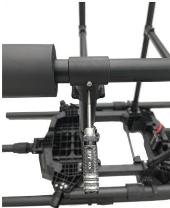
5. Install the diagonal brace: Insert the straight tee into the inclined aluminum tube, and fix all the screws of the straight tee.
