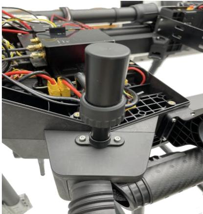
17、 Finished RTK antenna installation.
