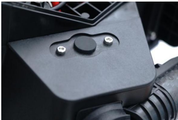
13、 There are reserved holes for the RTK antennas at both ends of the front fuselage.
