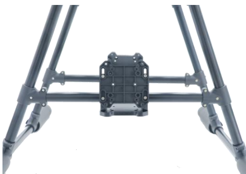
7、 The radar fixing plate installation : install the adapter plate on the tripod diagonal support.
