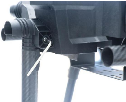
7、 The front and rear arm fixed installation: Use round head M6*50 screws to fix the arm.
