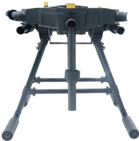
9.The finished front and rear arm fixed.
