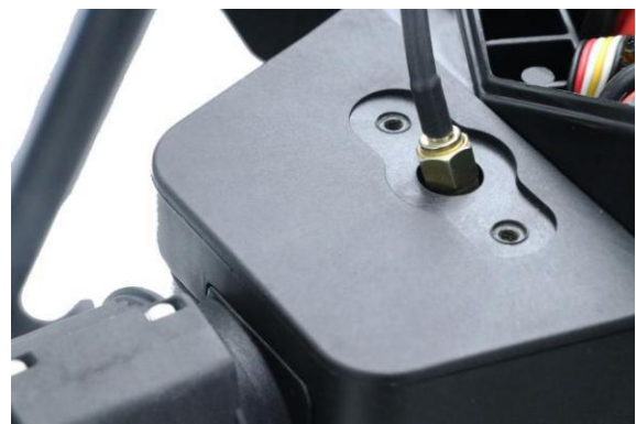
14、 The RTK antenna needs to pass through the reserved hole to reach the flight control compartment.
