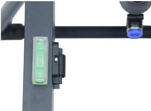
7、 Calibrate the body horizontally. Adjust the body level until the display is centered. If it is not level.
