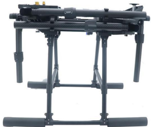
10.The finished front and rear arm fixed.
