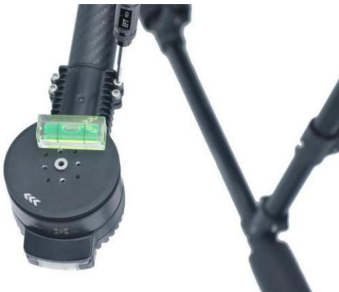
8、 Fully unfold the arms after adjusting the fuselage, tighten the nuts, and perform horizontal motor calibration. The calibration method is the same as that of the fuselage, and fix the motor screws.
