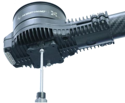
4、 Install the X6 adapter on the body and fix it with M3*8 screws.
