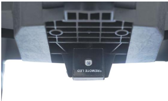
15、 The LED light installation: Use 3M glue to fix the LED light on the patch position at the bottom of the tail.
