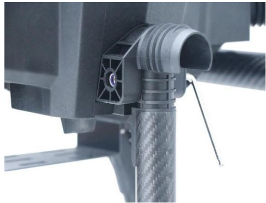
8、 The front and rear arm fixed installation: Use M6 locknut to fix the reverse side.
