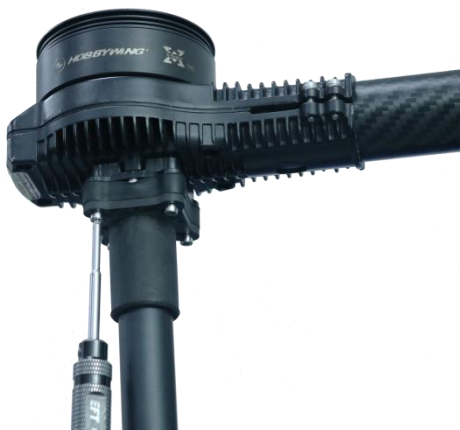
5、 Fix the print head on the X6 adapter and fix it with M3*16 self-tapping.
