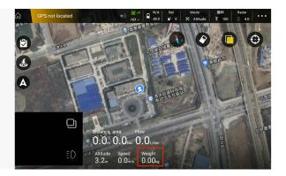
If the weight is inaccurate after changing the barrel or after a period of continuous use, tare calibration and weight calibration can be performed through the software to ensure the accuracy of the weight data.
