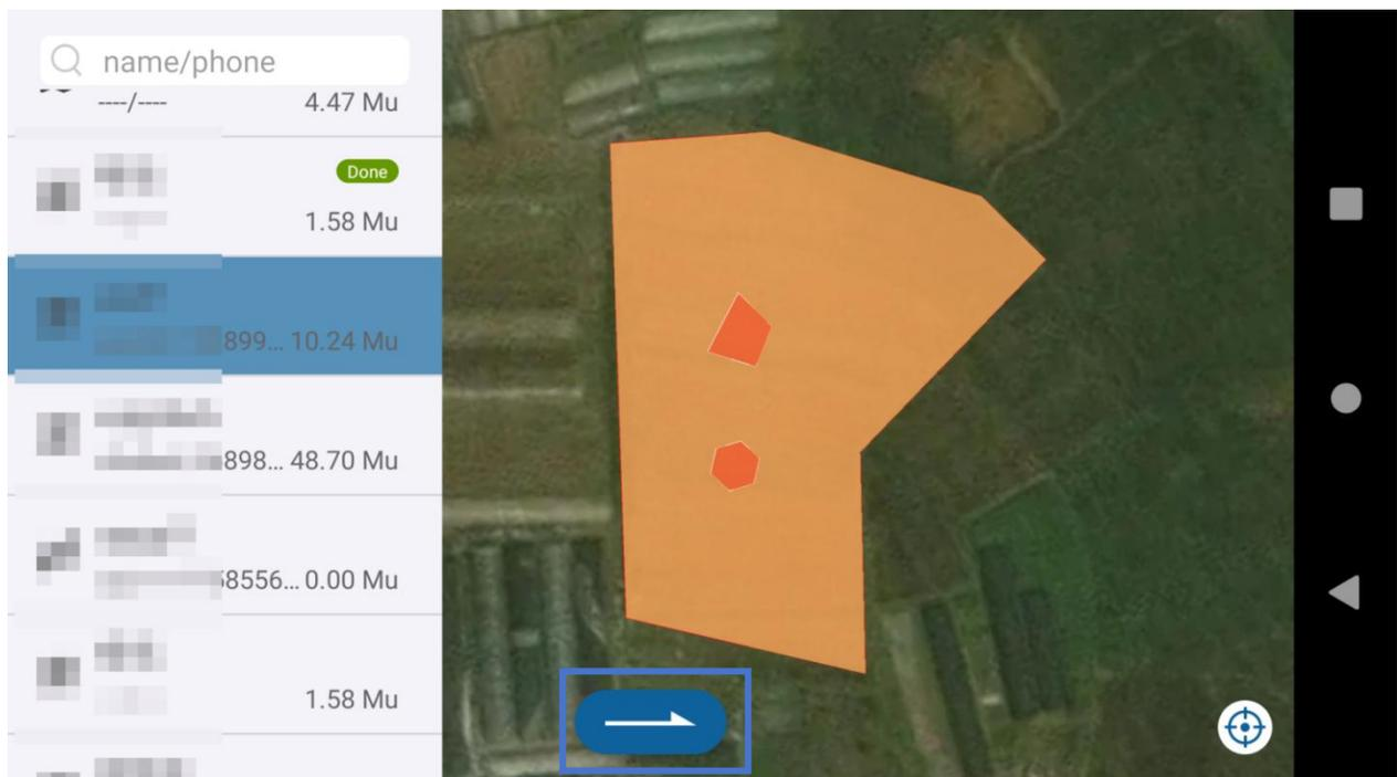
c . Tap one of the plot corner on the map to set the starting point. The Route Width, Route type, Maximum mileage, Safety Dis and Obstacle safe Dis accordingly.
